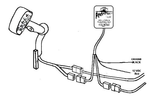
To Install the Peek-a-boom PB3 In later Rogators, simply follow the control wiring from the control stick to the connector as shown above. Separate the connector and install the connectors from the PB3 as shown, being sure to match the correct gender plug to each. As long as the pairs match, the connection cannot be made incorrectly.
